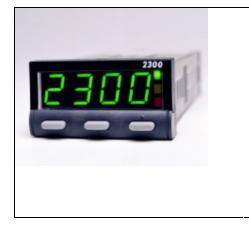
The 2300 is available as an indicator or controller. Small size does not come at the expense of features, they have large 10mm high displays, 2 amp relays and full 3-wire PT100 inputs. The controller features our hands-free Easy Tune PID algorithm.
