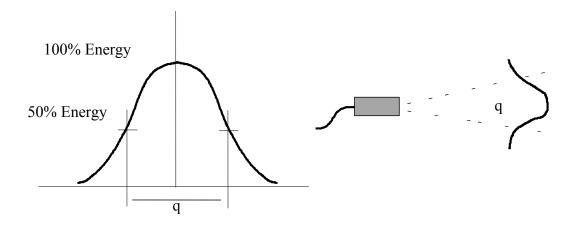
The other popular definition of Field of View is the "90% of Energy." This definition is more common in non-IR devices, but has been growing in its acceptance over the past ten years. This method defines the Field of View as the angle where 90% of the integrated energy of the bell curve found from an optical rotation experiment. See drawing:
