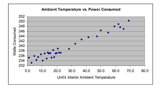
We have determined some average power consumption for SmartIRt/c<sup>™</sup> model types. These averages were determined using a very small sample size. Additionally, component batches have a big effect on the power consumed, so many units produced in a year might not have the same average. Always follow the maximum consumed power specification.
