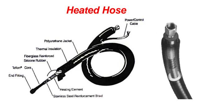
Heated Hose from Heaters Controls & Sensors is manufactured with high quality Teflon hose that are FDA and CSA approved. Heated Hose has a smooth Teflon Core which is electrically heated for continuous operation to high temperatures of 450° F (232°C).
