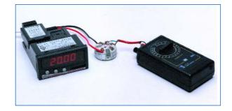
TYPICAL SET-UP The above picture shows FUZ 77 TC, Indicator, and Thermocouple simulator.
