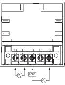
When a time switch and load power supply are the same
